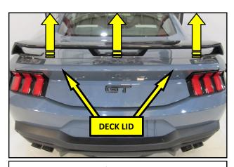
**13.** Remove the spoiler from the decklid and set it aside. Use a rubber eraser wheel and a drill to remove the adhesive from the deck lid.
