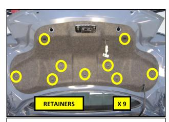
**4.** Using a panel trim removal tool, pry the 9 retainers from the liner.
