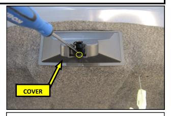
**2.** Remove Using a small screwdriver, pry the bottom of the truck latch cover away from the latch and remove it from the vehicle.
