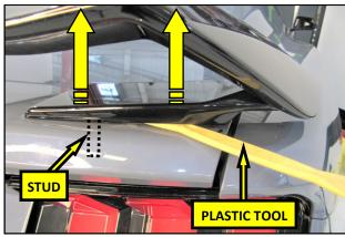
**12.** When the adhesive has fully softened, carefully pry the spoiler off of the decklid using plastic trim tools. **Note:** The OEM spoiler has locating studs under each section in contact with the decklid. Work the tools around these studs to separate the spoiler from the vehicle.
