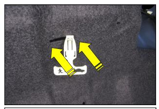
**5.** Push the release handle through the opening in the liner.
