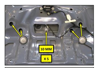
**10.** Using a 10 MM socket, remove the five flange nut in the trunk lid. **NOTE:** Special care should be taken to avoid dropping the nuts into the trunk lid.
