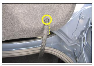
**6.** Pull the wiring harness out of the liner and remove the liner from the vehicle.
