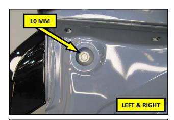
**9.** Using a 10 MM socket, remove the bolts from both ends of the trunk lid and lower the trunk lid.
