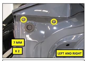
**7.** Using a 7 MM socket, remove the two screws on both sides of the trunk lid.
