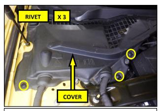
**1.** Raise the hood of the vehicle. Using a trim panel removal tool, remove the three plastic rivets in the battery cover and remove the battery cover from the vehicle.
