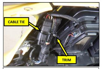
**15.** Secure the Sub Harness wiring to the vehicle using a cable Tie (Not Included). Trim the excess length.
