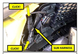
**14.** Connect the Sub Harness, in line, with the RTR Light and the OEM harness, as shown. Verify that all of the harness connectors are positively engaged with the mating connector.
