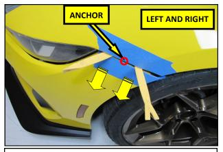
**7.** Using plastic trim pry tools, carefully separate the bumper cover from the fender. **NOTE**: There is a single fir tree anchor in the cover that will need to be pried out of the fender.
