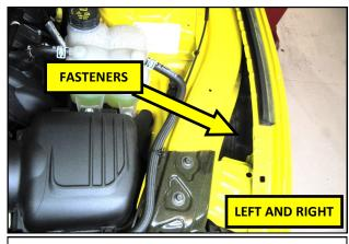
**5.** Locate the inner fender fasteners securing the bumper cover to the fenders.
