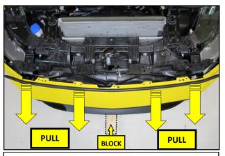
**12.** Lift the bumper cover up and over the core support posts and pull it forward, exposing the back side of the Grille and Lights. Allow the bumper cover to rest on the block or blocks from step **11**.
