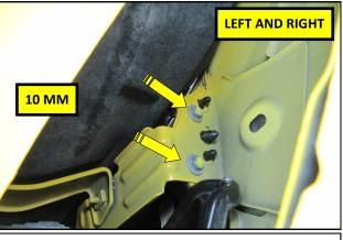
**18.** Using a 10 mm socket, reinstall the two OEM bolts to secure the bumper to the fender. Repeat this step on the opposite side of the vehicle.
