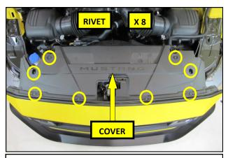
**8.** Using a panel clip removal tool, remove the eight plastic rivets in the core support cover.
