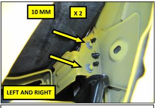
**6.** Using a 10 mm socket, remove the two flange bolts securing the bumper cover to the fender. Use caution when removing the bolts and take care not to drop them.
