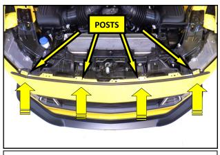
**16.** Lift the bumper cover back onto the vehicle and hang it using the core support posts.
