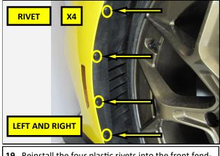
**19.** Reinstall the four plastic rivets into the front fender liners and cover. Repeat this step on the opposite side of the vehicle.
