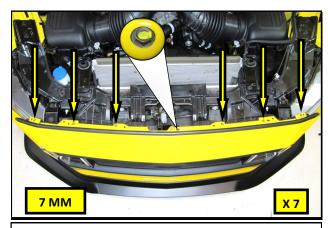
**20.** Use a 7 mm socket to reinstall the seven OEM screws along the upper bumper cover. Tighten the screws by hand to avoid over damage to the core support.
