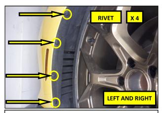
**3**. Turn the front wheel inward as shown. Using a trim panel removal tool, remove the four plastic rivets in the fender liner. Repeat step **3**. on the opposite side of the vehicle.
