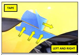
**4.** Place a layer of protective tape above and below the gap between the bumper cover and the fender. Repeat step **4.** on the opposite side of the vehicle.
