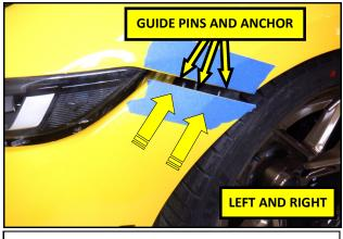
**17.** Lift the bumper cover up and press the fir tree anchor and guide pins into the fender. Remove the tape when the two halves have been joined.
