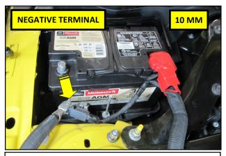
**2.** Using a 10 mm socket, loosen the negative battery terminal on the battery and disconnect the terminal, as shown.
