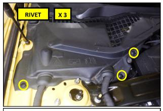
**24.** Reinstall the battery cover and secure it using the three plastic rivets removed in step **1**.
