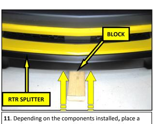
**11**. Depending on the components installed, place a wooden block or two, under the front edge of the bumper cover/chin splitter as shown.
