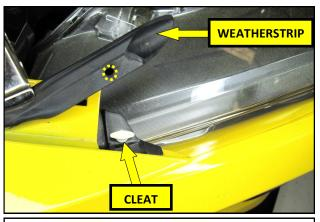
**21.** Carefully reattach the weatherstrip foam onto the cleats on each side of the vehicle.
