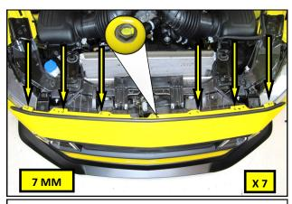
**10.** Using an 7 mm socket, remove the seven screws along the upper bumper cover.
