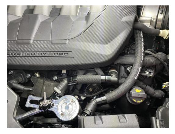
**8.** Install the vacuum hose from the catch can to the intake manifold vacuum fitting. Be sure the arrow printed on the check valve is facing away from the catch can, towards the engine.
