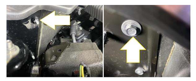
2. Install the 6mm x 25mm bolt, lockwasher, washer in place of the bulkhead bolt and tighten it.
