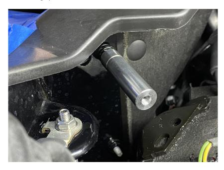
**4.** Install the bracket extension and 90 degree bracket using the supplied 6mm x 50mm long bolt. Be sure the short side of the 90 degree bracket is facing up. Tighten the bolt with a 10mm socket to secure the bracket.
